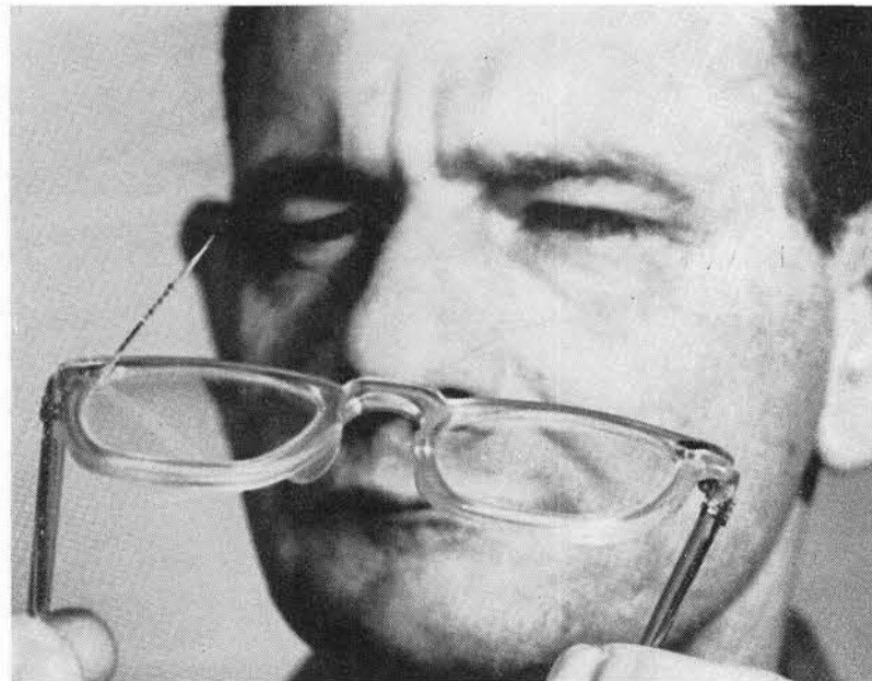
SAFETY GLASSES with wooden splinter tightly lodged between frame and glass are closely examined by Fred Hohmann (8222-2) who was wearing them when the sliver struck the glass and deflected. A circular saw sent the piece of plywood flying with enough force to pierce his eye, if it wasn't for his safety glasses.
